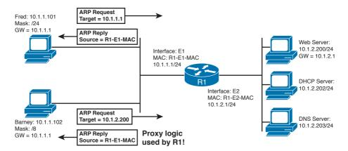
Figure 5-1 Comparing ARP and Proxy ARP
