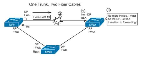
Figure 3-15 STP Problems with Unidirectional Links
