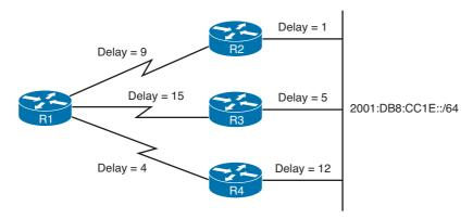
Figure 8-5 Sample Network Operating EIGRP in IPv6 Mode
