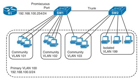
**Figure 2-2** *Switched Network Utilizing Private VLANs*
