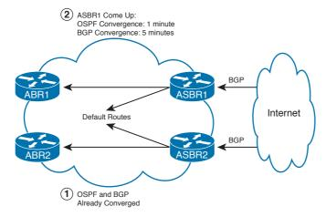
Figure 9-12 OSPF Stub Router
