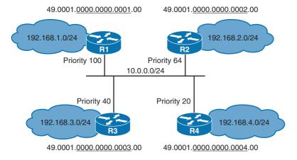
Figure 10-5 DIS Elections on a Broadcast Segment
