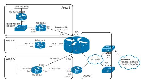
Figure 9-5 Network Used in LSA Examples
