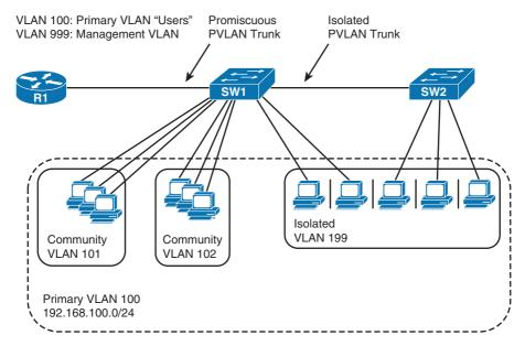
Figure 2-3 Switched Topology Utilizing Special Trunk Types
