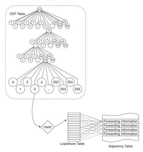
Figure 6-4 CEF Load Balancing
