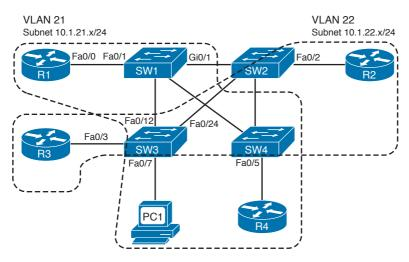
Figure 2-1 Simple Access and Distribution
