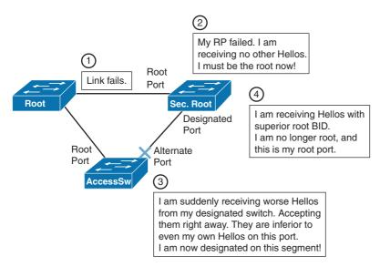
Figure 3-12 Accepting Inferior BPDUs from Designated Switch (Indirect Link Failure)
