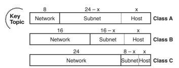
Figure 4-2 Formats of IP Addresses when Subnetting
