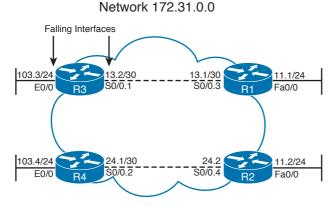
Figure 7-2 Sample Internetwork Used for Loop-Prevention Examples
