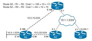
Figure 9-3 Single-Area SPF Calculation: Conceptual View
