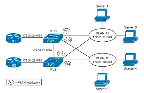
**Figure 6-7** Layer 3 Topology View: Example Using MLS
