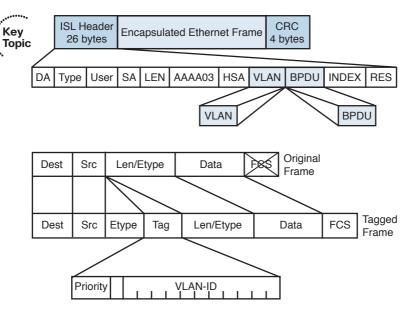
Figure 2-4 ISL and 802.1Q Frame Marking Methods
