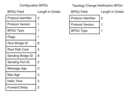
Figure 3-1 Format of STP Bridge Protocol Data Units
