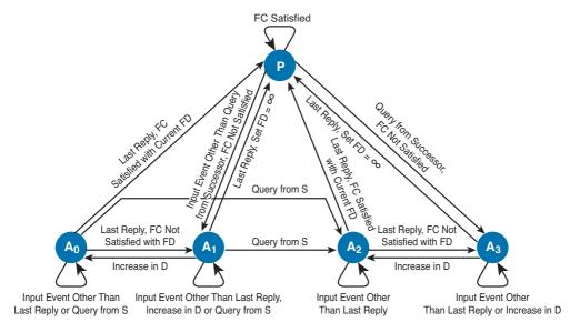
Figure 8-7 Diffusing Update Algorithm Finite State Machine
