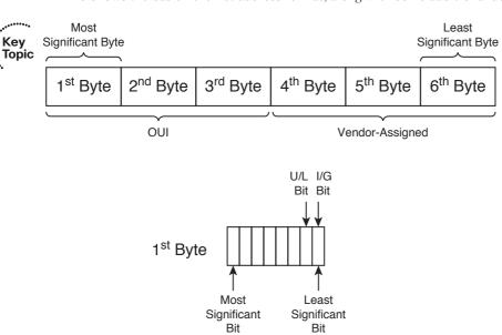
Figure 1-5 Ethernet Address Format
