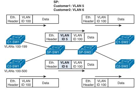
Figure 2-6 Q-in-Q: Basic Operation
