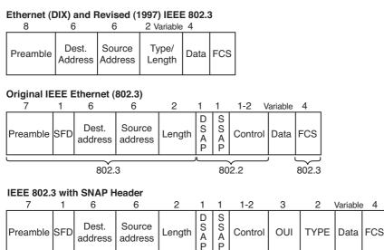
Figure 1-4 Ethernet Framing Options
