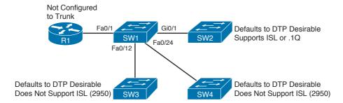
**Figure 2-5** Trunking Configuration Reference for Example 2-6
