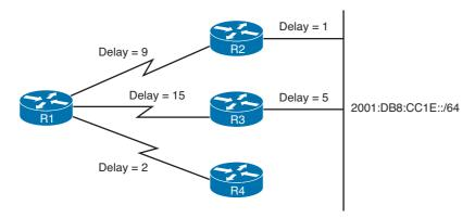
Figure 8-6 Modified Sample Network Operating EIGRP in IPv6 Mode
