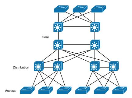
Figure 1-10 Typical Switch Network Design
