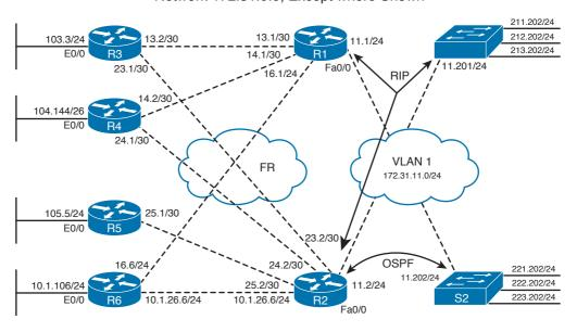
Figure 7-3 Sample Internetwork Used for RIPv2 Configuration Examples
