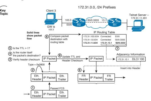
Figure 6-1 Forwarding Process at Router3, Destination Telnet Server
