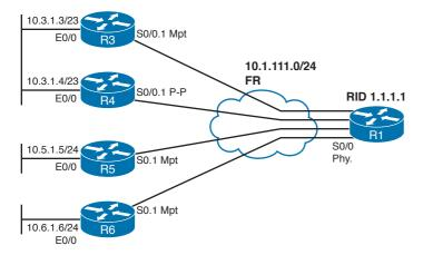
**Figure 9-2** Network Used in the Frame Relay Priority and Network Type Example Example 9-3 depicts the following scenarios relating to DR election in Figure 9-2:
