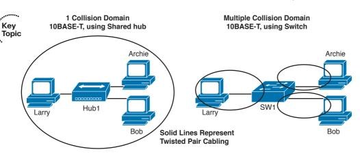
Figure 1-2 Collision Domains with Hubs and Switches
