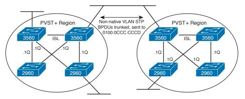
Figure 3-9 Network as Perceived by Non-VLAN 1 PVST+ STP Instances
