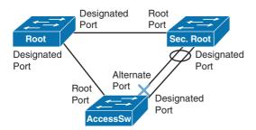
Figure 3-16 Permanent Switching Loop in a Misconfigured EtherChannel
