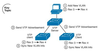
Figure 2-7 VTP Revision Number Basic Operation
