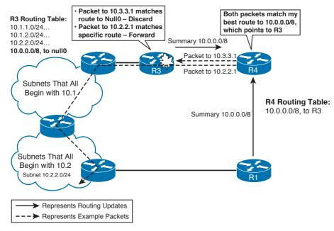
Figure 11-7 Route Summarization Suboptimal Routing and Routing to Null0
