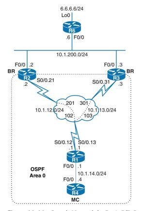
**Figure 11-11** *Sample Network for Basic PfR Configuration*
