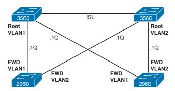
**Figure 3-6** Operation of PVST+ for Better Load Balancing
