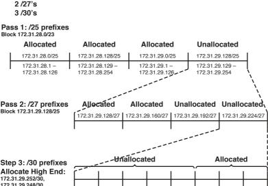
Figure 4-3 Example of VLSM Subnet Allocation Process
