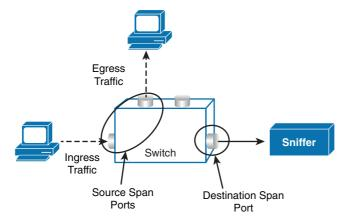
Figure 1-7 SPAN Topology
