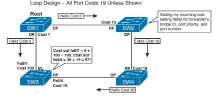
**Figure 3-3** Calculating STP Costs to Determine RPs
