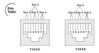
Figure 1-1 RJ-45 Pinouts with Four-Pair UTP Cabling
