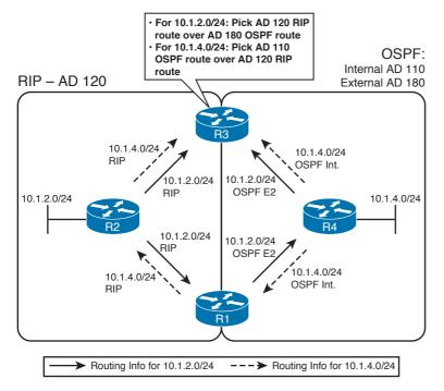
Figure 11-5 Effect of Differing ADs for Internal and External Routes
