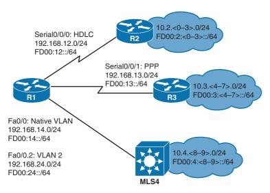
**Figure 6-3** Example Network Showcasing CEF Operation
