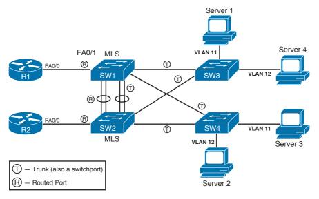
Figure 6-6 Physical Topology: Example Using MLS
